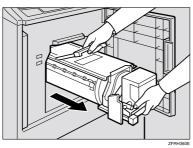
**5** Remove the drum unit from the machine while holding the upper drum stay.
